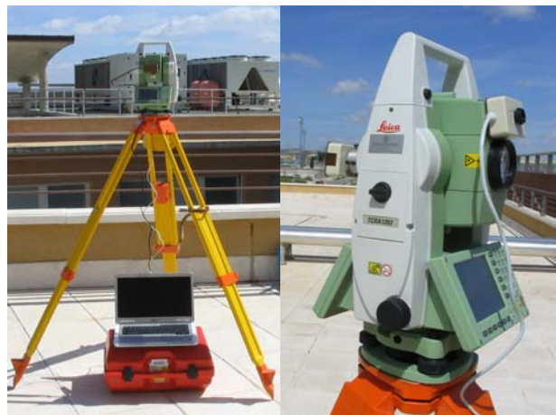
Figure 1. Left: Prototype of sensor system. Right: cameras coupled to the total station.
