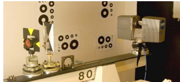
Figure 4. Measurement at a first distance about 1 m from the laser scanner. The tubular level that was used for levelling the sled is also shown in the image. Circles seen on the wall were not used in this calibration.
