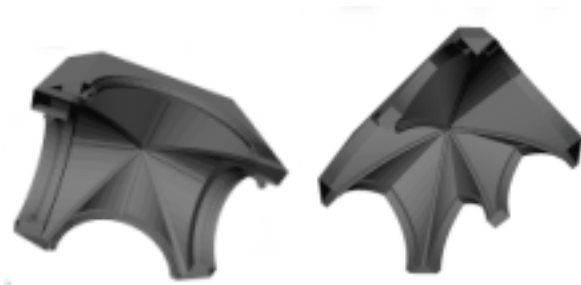
Figure 2: The architectural model is a vault: the number of arches and their heights are different in the two instances.
