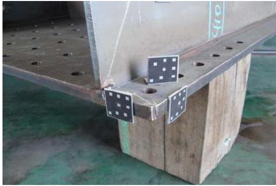
Figure 14. Target setting for corner point measurement using field calibrated target
