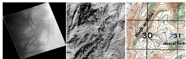
Figure 2.2 Provided cartographic data (Left: DEM, Middle: satellite orthoimage, Right: topographic map). The outline in left figure is referenced to the area of satellite orthoimage, and it is also the range of FJHP.
