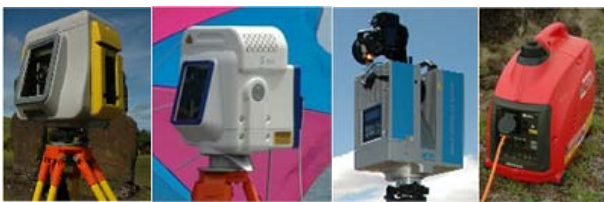
Figure 1. Terrestrial laser scanner Trimble GX (used in 2007), Trimble GS101, IMAGER 5006 from Zoller & Fröhlich (both used in 2008), and Honda power generator
