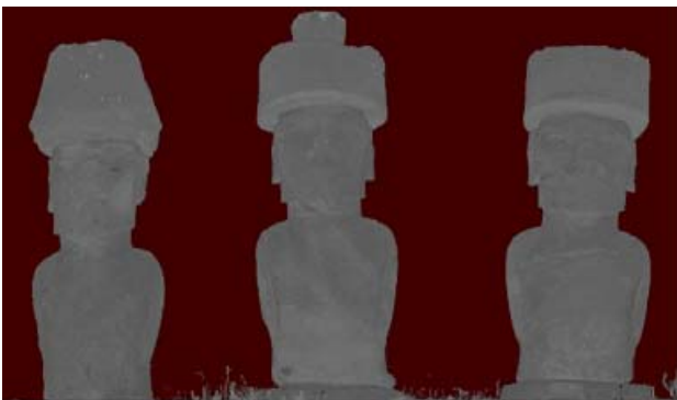
Figure 5. Representation of point cloud with intensity values, which were scanned from one scanner station at Ahu Nau Nau with the terrestrial laser scanning system Z+F IMAGER 5006
