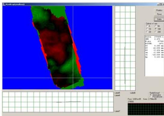
Figure 9 b. Spatial distribution of relative deviations after final plate stone 'A' (black colour–good matching, green and red colours decreased accuracy of matching).
