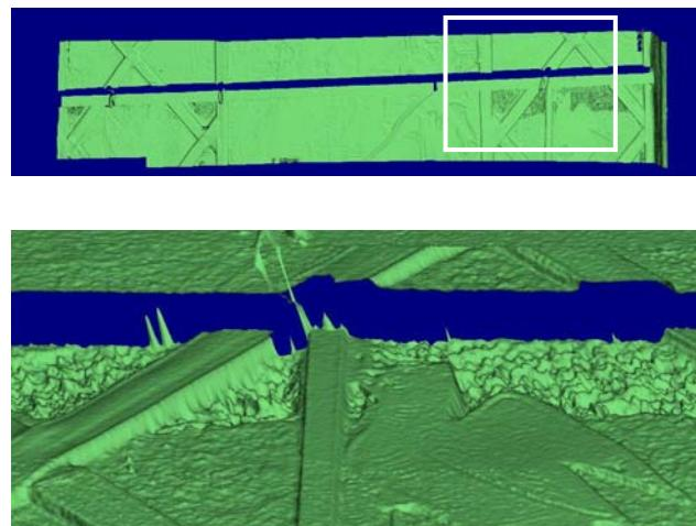
Figure 5. Zoom in of noise enhanced in a partial model of the window, probably caused by presence of a metal scaffolding behind the glass
