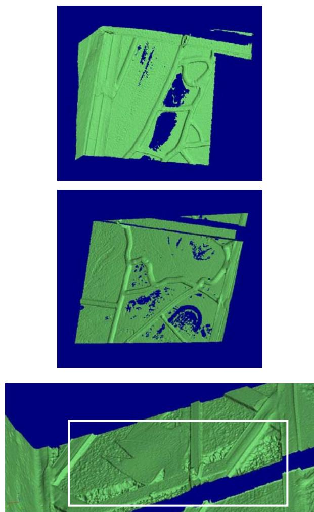
Figure 4. Details 1 and 2 from Fig. 3, showing lacunas, interpreted as a combination of more factors. Detail 5 showing its thickness with respect to the surrounding glass
