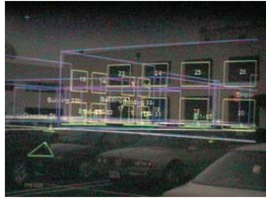
Fig.3 BARS shows the interior construction of a building by this system
