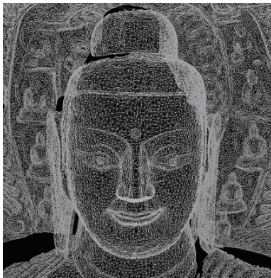
Fig.5 Digital triangular model of head part in No.20 grotto
