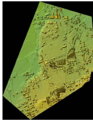
Figure 4. Gradation map by last pulse data (Oorui)
