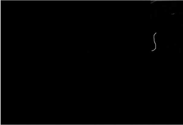
Figure 6. Images difference after precise cross-correlation: the crack is isolated
