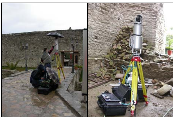
Figure 7. Laser scanning surveys.
