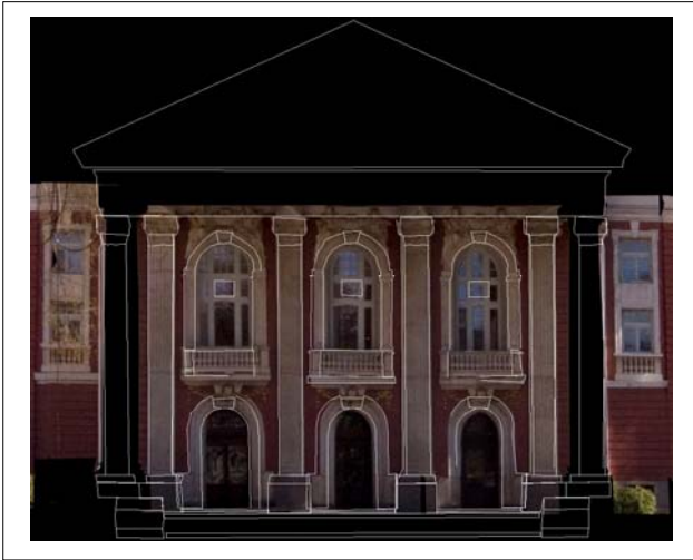
Figure 5. Rectified mosaic of front entrance facade.
