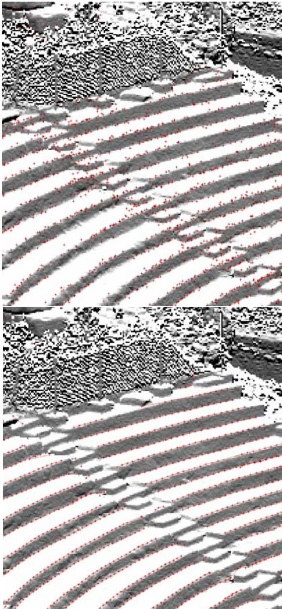
Figure 5: Shading of the 2.5D surface model derived from the polar observations overlaid with vector data; Upper image: automatically extracted start-segments (every twentieth TLS point was analysed); Lower image: automatically extracted feature lines with the proposed approach.
