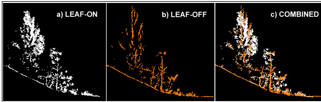
Figure 5. Section through TLS datasets during a) leaf-on, and b) leaf-off conditions. Differences are highlighted through combination (c).
