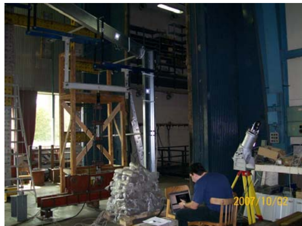
Figure 8. Laserscanning station, note the tilted scanner head and the reflectors on the portal frame
