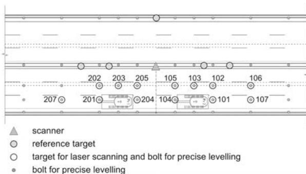
Figure 5. Measurement setup for terrestrial laser scanner and targets for TLS and precise levelling.
