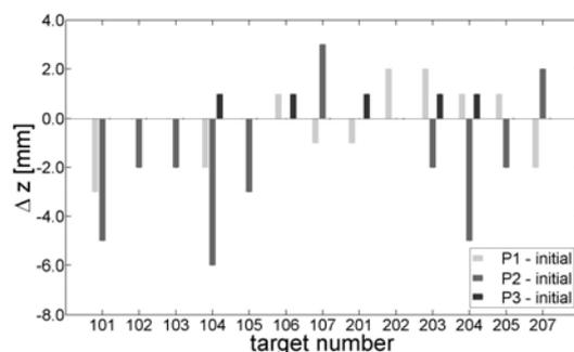
Figure 7. Vertical displacements of sphere centres between different loadings and initial situation measured by terrestrial laser scanner Imager 5006.
