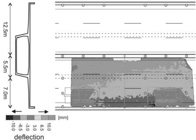
Figure 6. Deflections of cantilever slabs detected by terrestrial laser scanner (residuals of the scan points of loading P2 to the initial situation).
