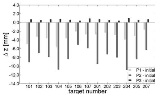
Figure 9. Vertical displacements of sphere centres between different loadings and initial situation measured by precise levelling.
