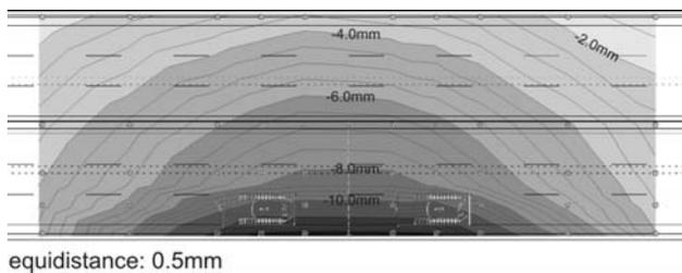
Figure 8. Deformations between initial situation and loading situation P2 of bridge girder detected by precise levelling.
