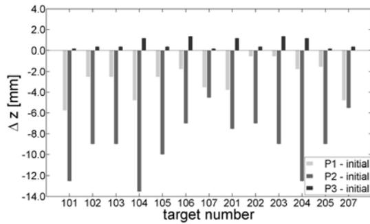
Figure 10. Transformed vertical displacements of sphere centres between different loadings and initial situation measured by terrestrial laser scanner.
