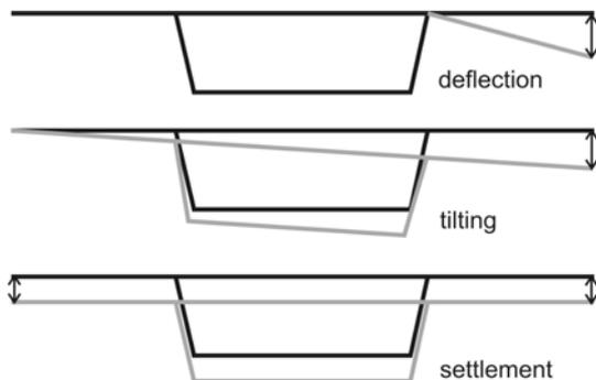
Figure 2. Expected deformation behaviours of the cantilever slabs and bridge girder under loading.
