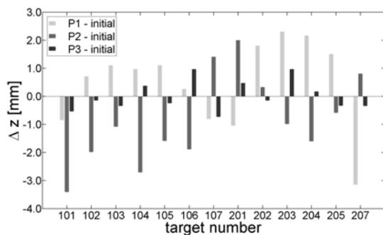
Figure 11. Differences between transformed vertical displacements of TLS and precise levelling for different loadings.
