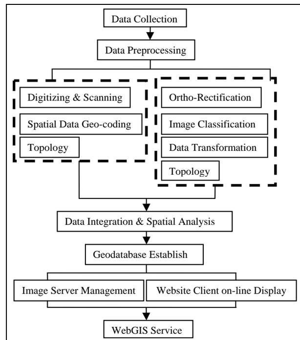
Figure 2. The flow chart of establishing geodatabase WebGIS
