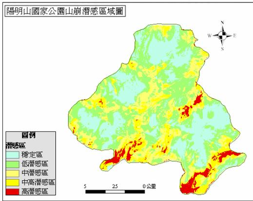
Figure 11. YMS National Park GIS Landslide Sensitive Layer
