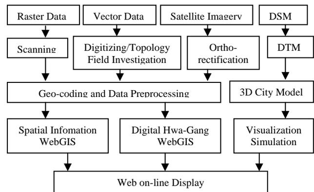
Figure 5. Procedure for Establishing Digital Hwa-Gang
