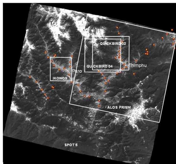
Figure 1. 60 x 60 km Bhutan testfield with 65 GPS-surveying GCPs.
