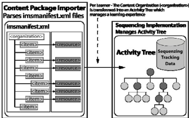
Figure 3: Relationships between a Content Organization and an Activity Tree. Adapted from: SCORM® 2004 3rd Edition Sequencing and Navigation, Version 1.0, p SN-2-4
