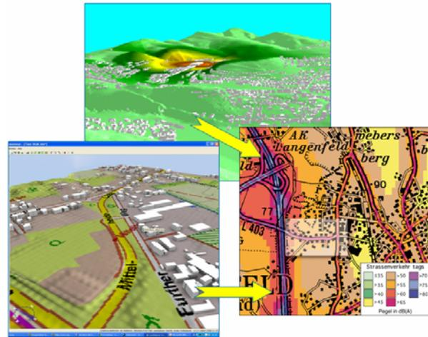
Figure 7: generation of noise pollution maps by noise dispersion simulation; result visualization using web services
