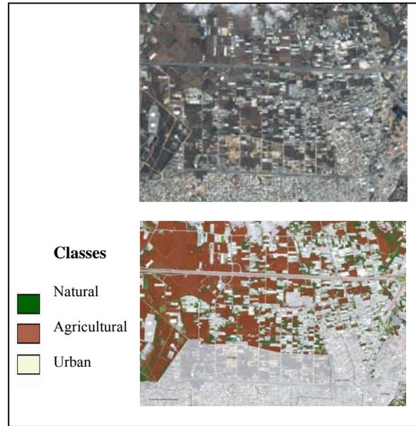
Figure 6. IKONOS orthoimage (up) from Thessaloniki and the corresponding classified (down) into three basic classes.
