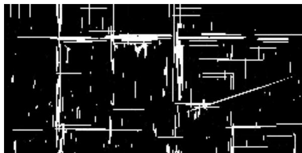
Figure 4. Result of road connection algorithm. The algorithm is based on road knowledge including continuity, shape, and topology of urban roads. The road features are obvious in the imagery.
