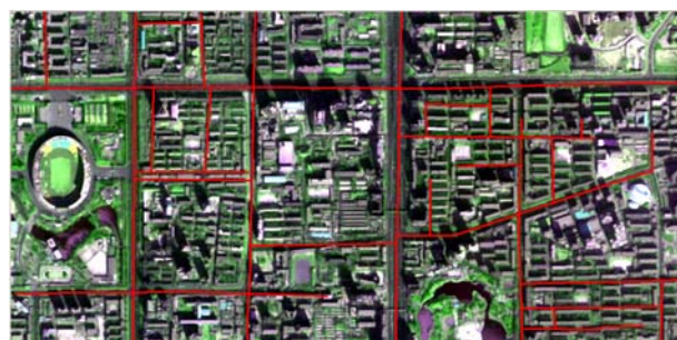
Figure 5. Compared image overlap road thematic image with the original image. It clearly shows the extraction result
