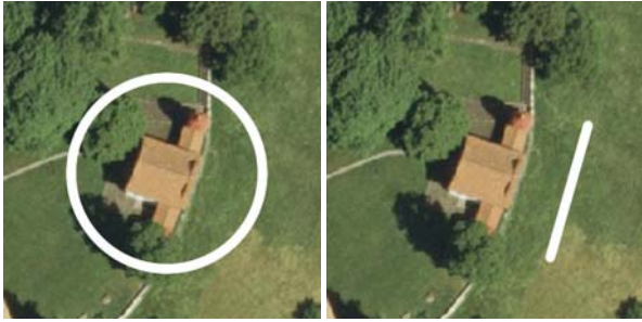
Figure 5: Flight Paths: Circle (left) and frontal stripe (Orthophoto: http://www.gis.ow.ch/ , 2008).
