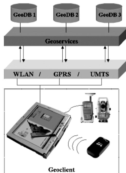
Figure4. Field based Mobile GIS architecture
