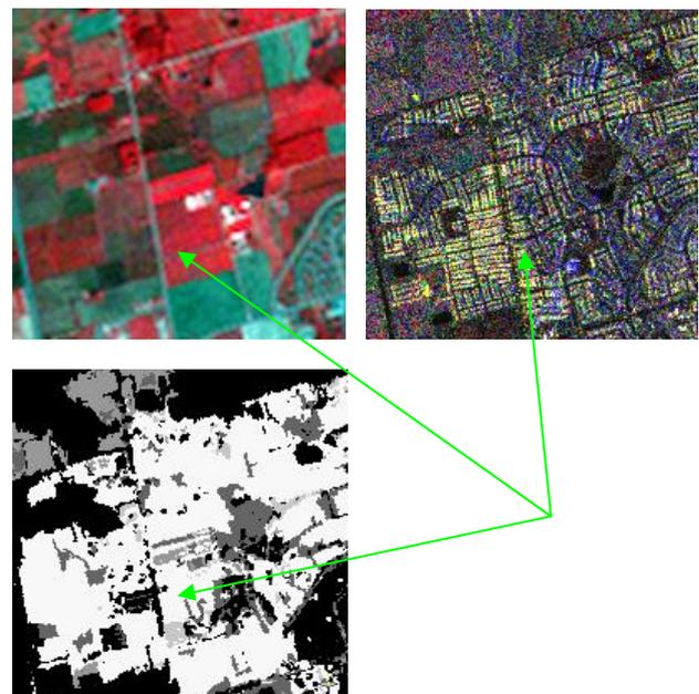
Figure 2. New built-up areas. Upper-Left: TM image, 1988; Upper-Right: SAR image, 2002; Lower-Left: Change map.
