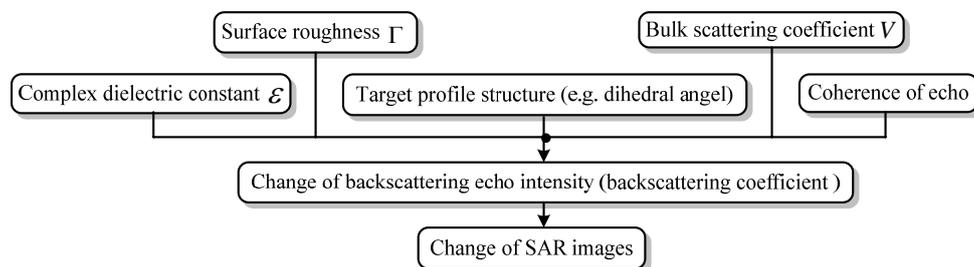
Figure 1 SAR image change factors from ground parameters
