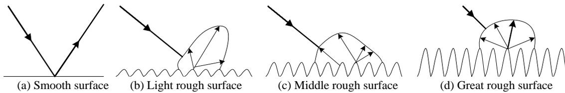
Figure 2 The reflection and scattering of different rough surfaces (Guo, 2000)
