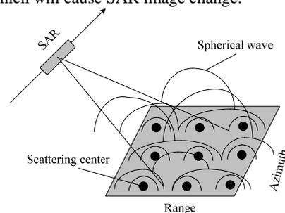
Figure 3 Coherent principle diagram of SAR imaging
