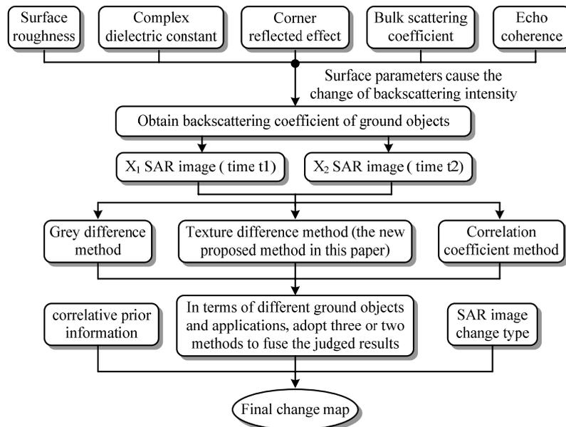
Figure 5 The flow chart of the integration SAR image change detection algorithm
