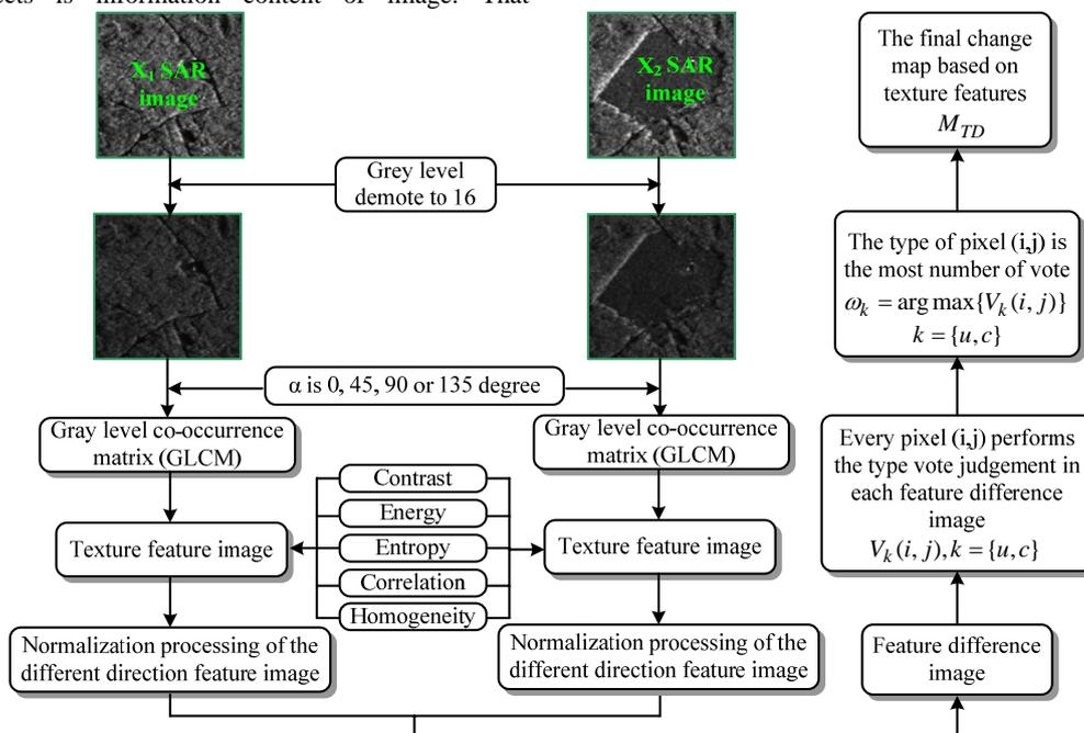
Figure 4 The change detection frame based on all texture feature fusion
