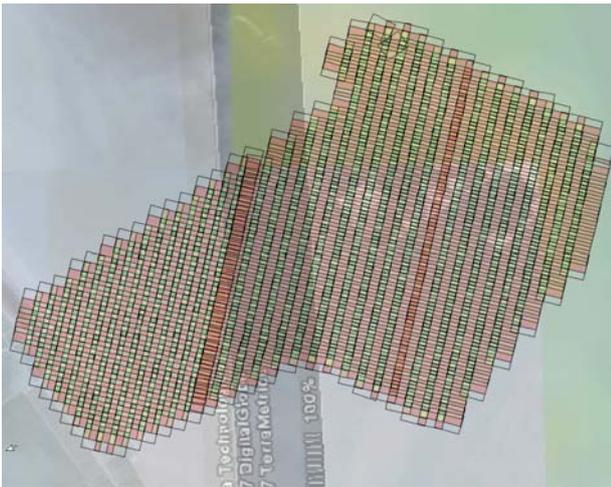
Figure 9: Footprints of a 220km<sup>2</sup> missions over an industrial area flown 900 m above ground (120 mm GSD)
