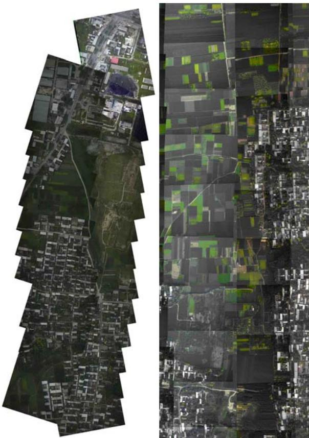
Figure 8: The left image block shows data captured without stabilization, on the right with stabilization
