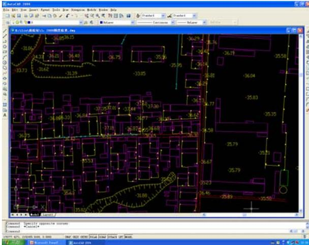
Figure 11: Digital map in scale 1:500 that has an accuracy between 5-10 cm
