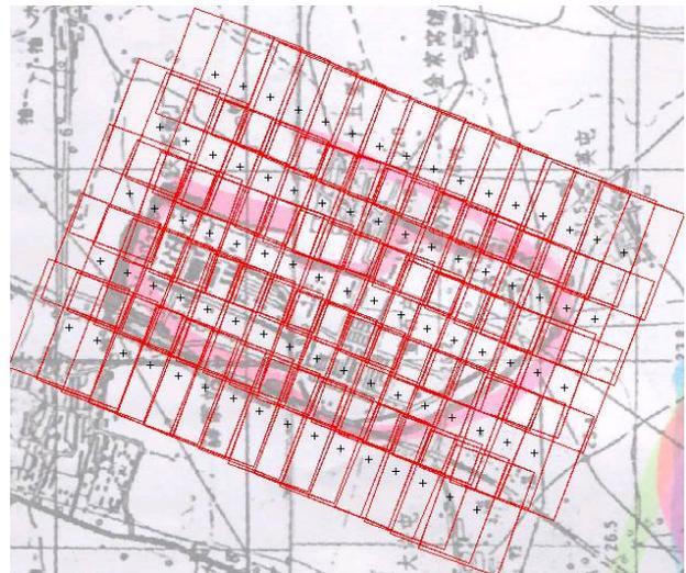
Figure 9: Footprints of a 6km<sup>2</sup> missions over a village flown 610 m above ground (82mm GSD)
