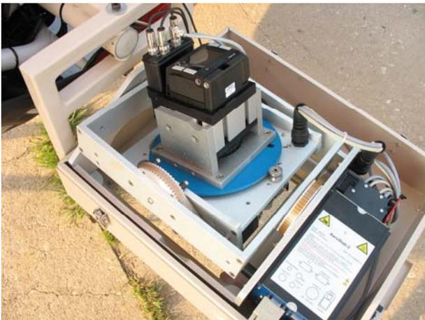
Figure 3: Rollei digital aerial camera with the AeroStab-2
