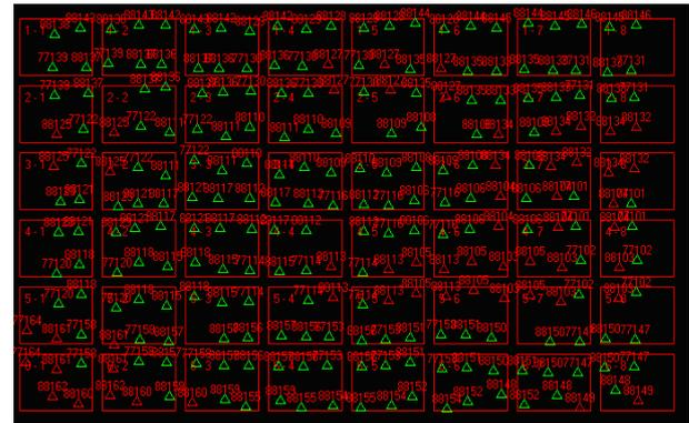
Figure 10: Scheme of a Tie- and Passpoint distribution for a small project during Automated Aerotriangulation
