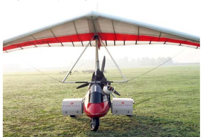
Figure 1: Microlight-Trike as a platform for aerial surveying using Rollei AIC, AeroStab-2 and AeroTopoL FMS
