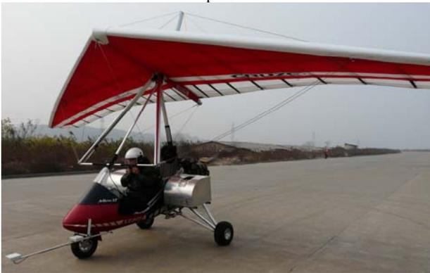
Figure 7: Trike ready for take of with the enhanced antennas for a stabile heading determination
