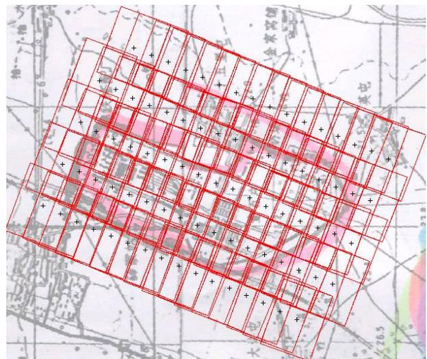
Figure 9: Footprints of a 6km² missions over a village flown 610 m above ground (82mm GSD)
