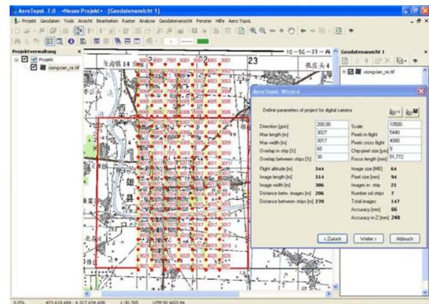
Figure 6: Xiongxian Testsite with the planned mission and the resolution, scale and expected accuracy
