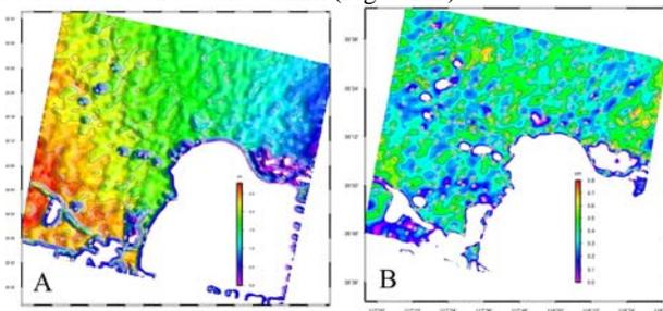
Figure 2. Comparison of tropospheric delay along radar line of sight between before and after removing baseline errors with curvature surface fitting method
