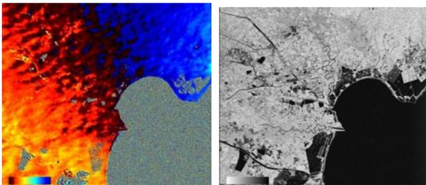
Figure 1. Tandem differential interferogram (left) and coherence (right) in Tianjin region
