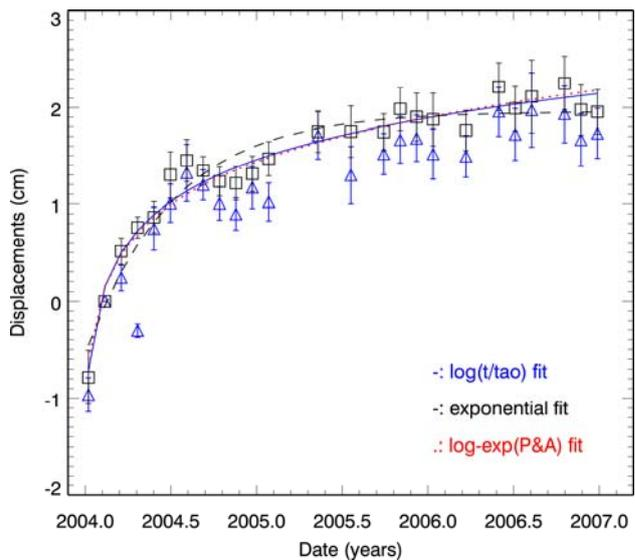
Figure 6. InSAR time series of averages for rapid uplift region B (2 km × 2 km, red and black squares in Figures 4 and 5 respectively). Note: (1) errors were estimated from RMS of the area of interest; (2) Blue triangles represent time series without MERIS water vapour correction whilst black squares indicate time series with MERIS water vapour correction.
