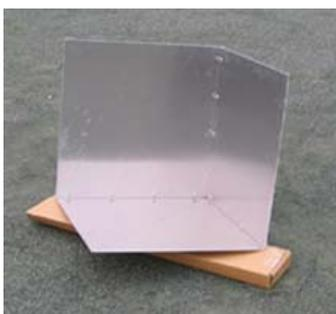
Figure 2. Corner reflector used in this study.
