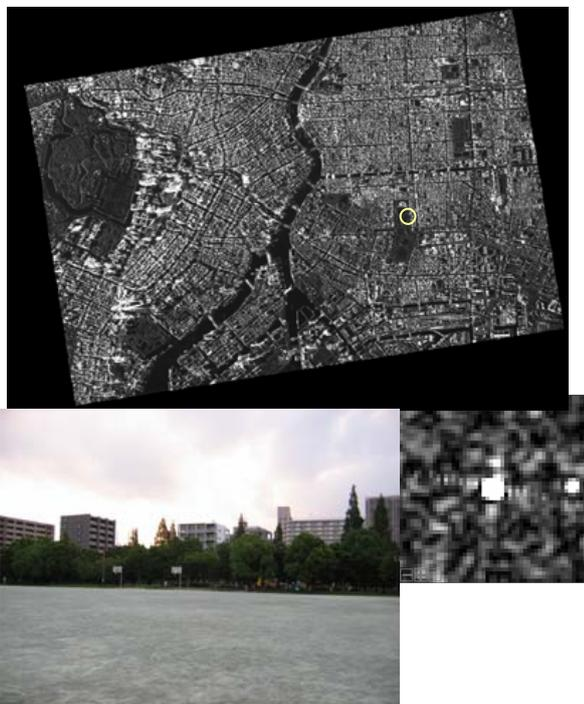
Figure 1. TerraSAR-X EEC product of Tokyo on 29<sup>th</sup> Nov., 2007 and an enhanced portion of the corner reflectors.
