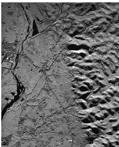
Figure 7. The image that filtered by Adaptive Lee local statistics
