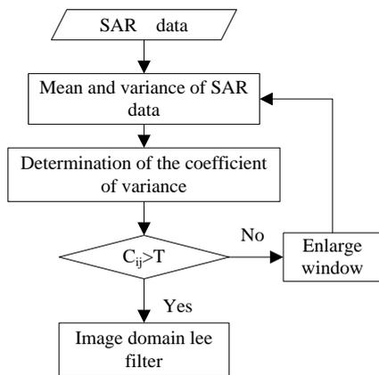
Figure 6. The routine of adaptive windowing algorithm
