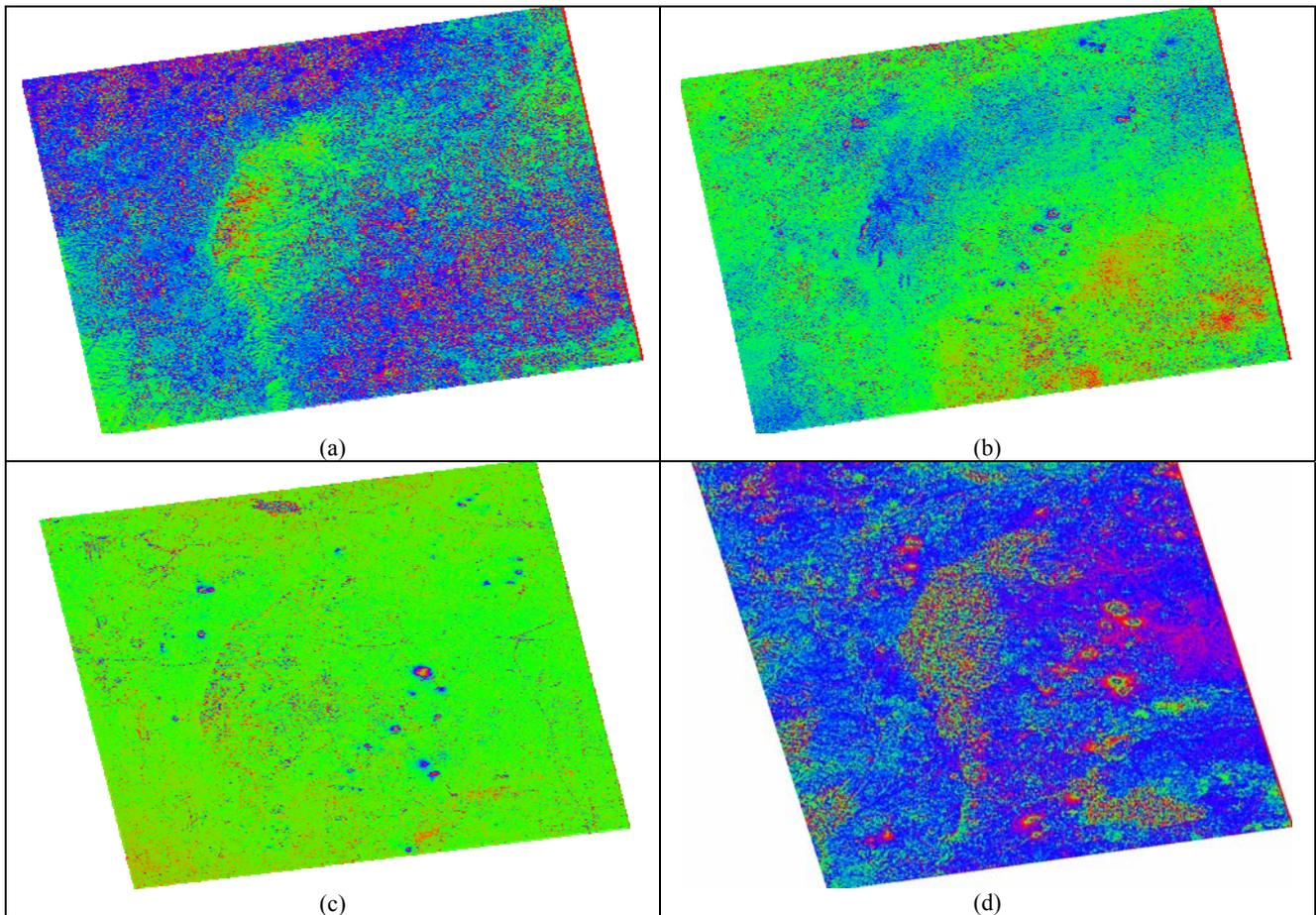
Figure 3. DInSAR interferograms of (a) – (c) ALOS interferometric pairs: 14/6/2007 - 30/7/2007 Bperp = 515m, 30/7/2007 - 14/9/2007 Bperp = 143m, and 15/12/2007 - 30/01/2008 Bperp = 351m, and (d) ENVISAT pair: 3/1/2008 - 7/2/2008 Bperp = 361m respectively.
