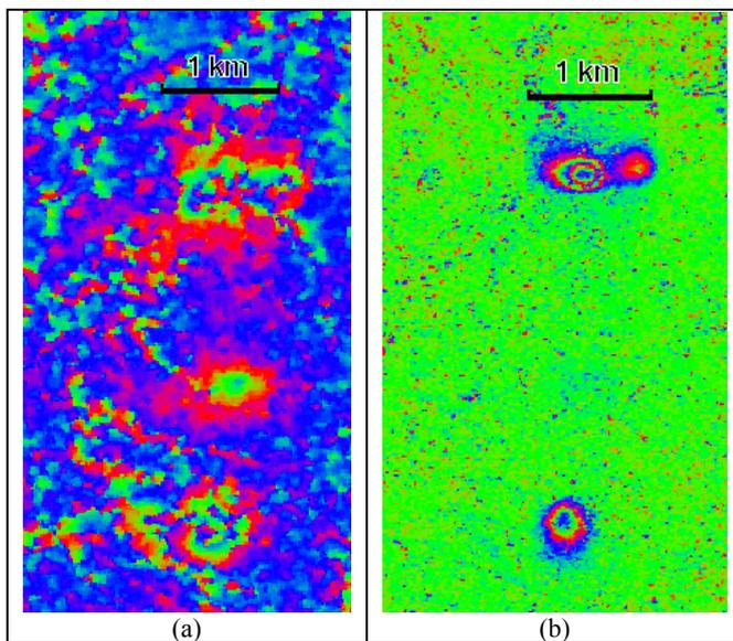
Figure 2. Enlarged DInSAR phase fringes induced by ground deformation of (a) ENVISAT (C-band) pair: 3/1/2008 - 7/2/2008 Bperp = 361m, and (b) ALOS (L-band) pair: 15/12/2007 - 30/01/2008 Bperp = 351m.
