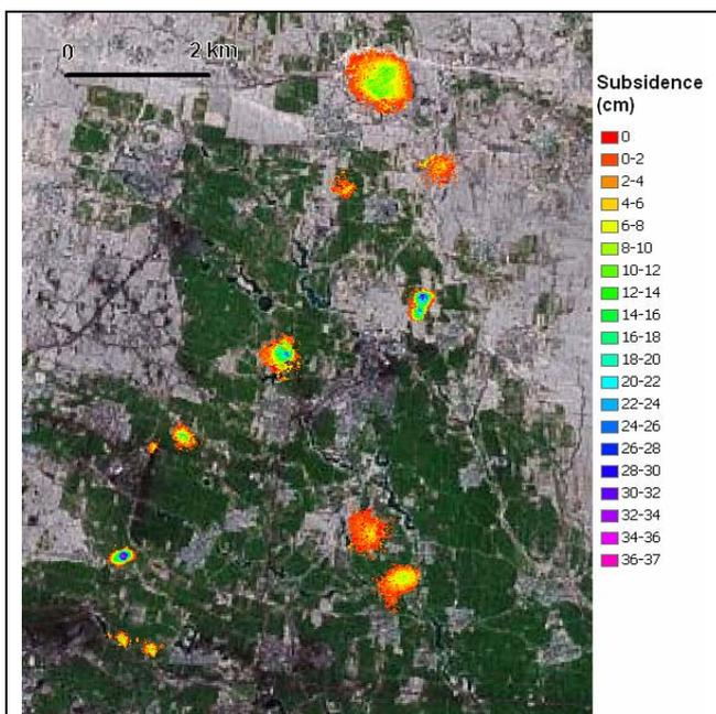
Figure 4. Ground deformation map derived from the ALOS interferometric pair: 15/12/2007 - 30/01/2008, overlaid on an optical image.
