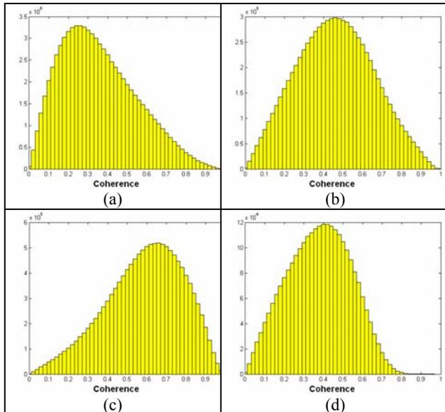
Figure 1. Histograms of coherence values of (a) - (c) ALOS interferometric pairs: 14/6/2007 - 30/7/2007 Bperp = 515m, 30/7/2007 - 14/9/2007 Bperp = 143m, and 15/12/2007 - 30/01/2008 Bperp = 351m, and (d) ENVISAT pair: 3/1/2008 - 7/2/2008 Bperp = 361m, respectively. The mean coherence value of these 4 pairs are 0.355, 0.461, 0.586 and 0.379.
