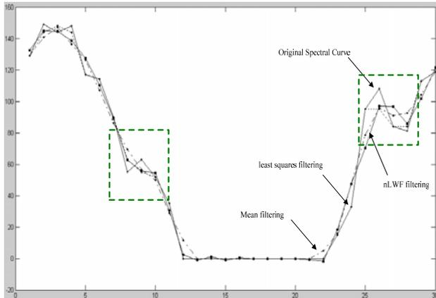
Figure 4 Different filtering result of spectral curve
