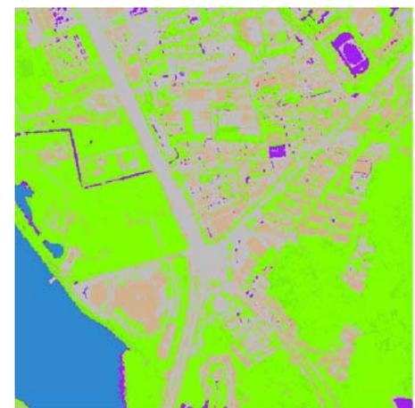
Figure.4 The fuzzy classification image from the combined NDVI image with multispectral QuickBird image
