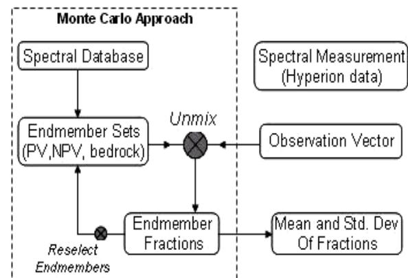
Figure1. Schematic diagram of AutoSWIR algorithm
