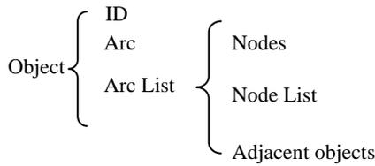
Figure 2. The structure of the vector data
