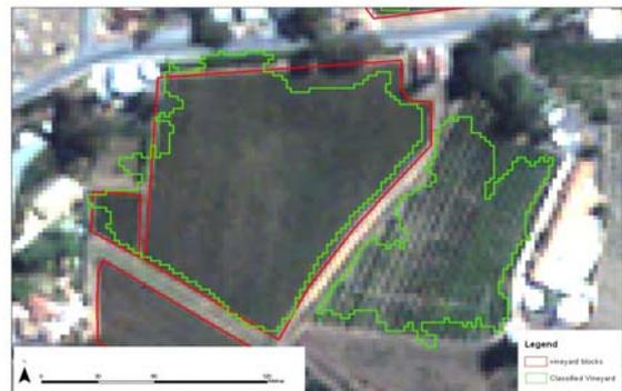
Figure 7. OOC of a sample vineyard using the QuickBird MS imagery. Red vector shows “truth”, the green the results of OOC. The green vector on the right corresponds to a non-vine horticultural crop.
