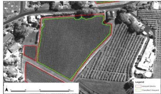
Figure 6. OOC of a sample vineyard using the QuickBird Pan imagery. Red vector shows “truth”, the green the results of OOC.
