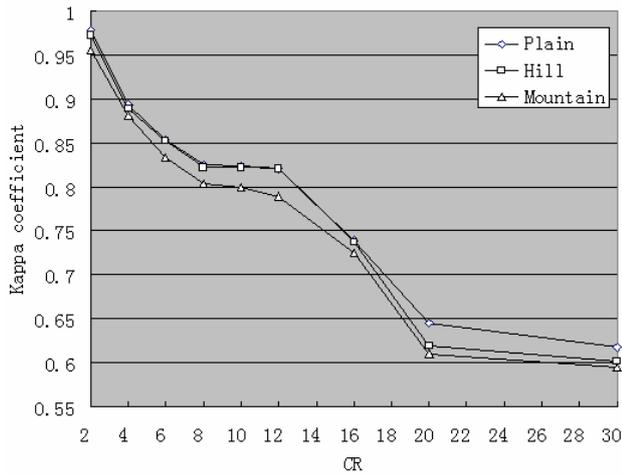
Figure 4. The relation between compression ratio and the Kappa coefficient (JPEG 2000)
