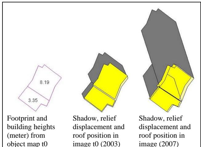
Figure 9. 3D building representation in a 2D map.
