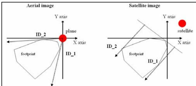
Figure 4. Difference in projection of relief displacement
