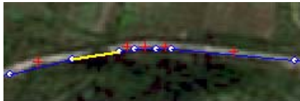
b. failure multi-scale template matching in shaded region
