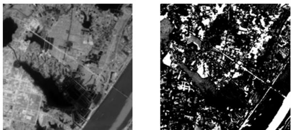
Figure 7. ICA-based change detection: background image IC1 and value changed image IC2
