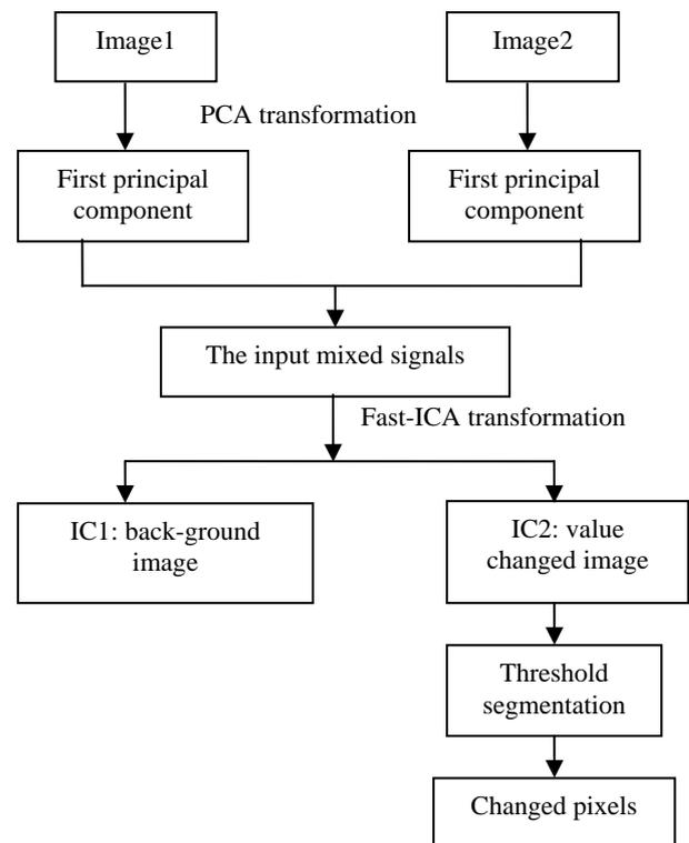
Figure 2. Fast-ICA based image change detection model
