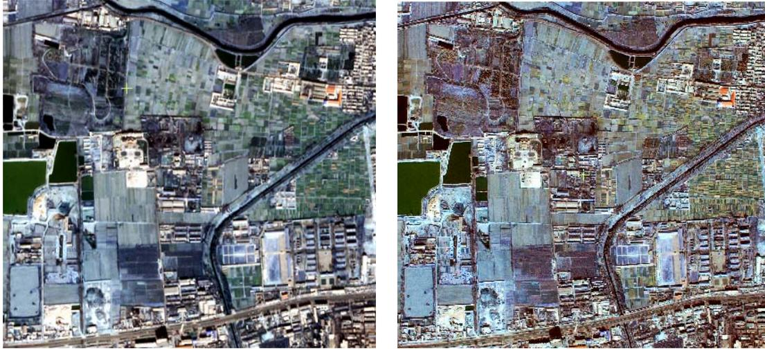
(a) Original multispectral, true color composite 441 x 413 (b) PCA fusion results, 1761 x 1649
