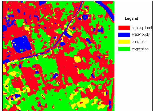
Figure 4. Classification result of SAR image based on multi-scale and multi-texture feature fusion and SVM (part of the test site)
