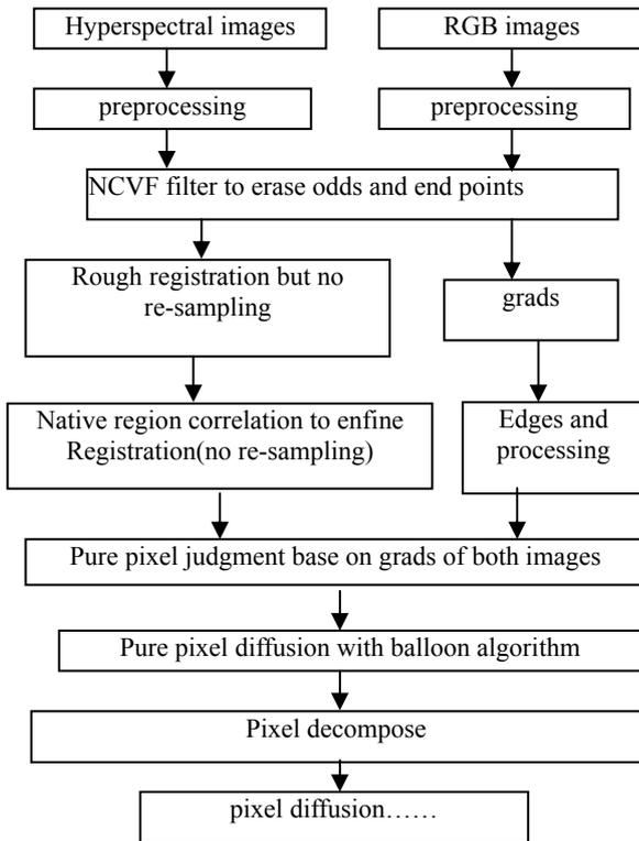
Figure 5. work flow of the fusion
