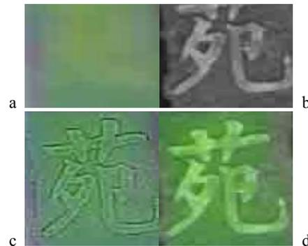
Figure 4 the low resolution image is blurred after register
