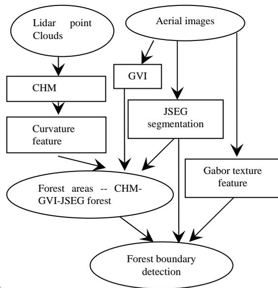
Fig. 8 Schematic workflow of overall process
