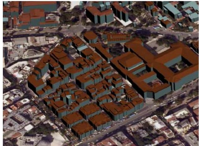
Figure 10. 3D city model of Istanbul Historic Peninsula as LoD2 in the Suleymaniye area superimposed on an orthophoto as an overview (top) and detailed view (bottom)
