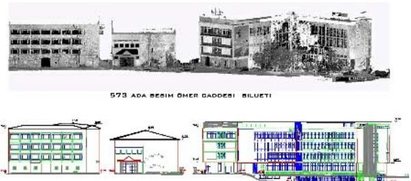
Figure 6. Detailed map of building façades using laser scanning data - laser scanning data (top) and façade plan (bottom)
