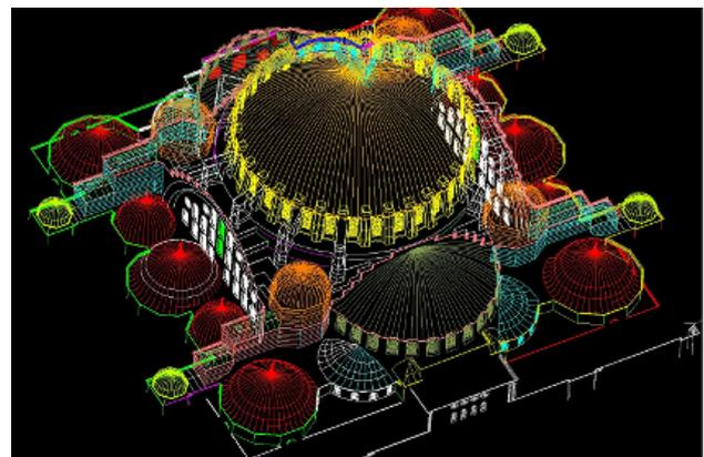
Figure 14. Wireframe of the Suleymaniye Mosque 3D model
