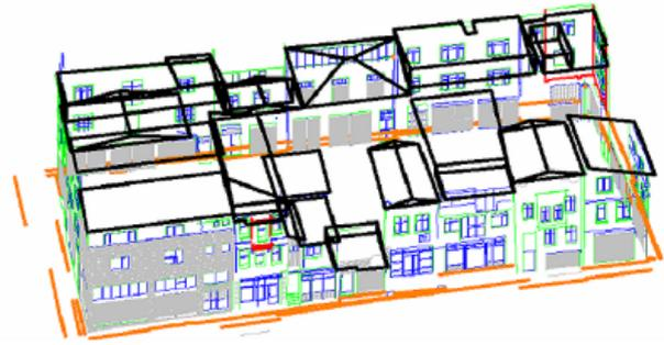
Figure 8. Combination of data from two different sources: 3D polylines of roofs based on aerial images and 3D polylines of facades from terrestrial laser scanning data
