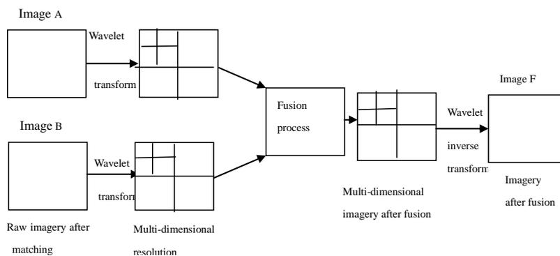
Figure2 Procedure of wavelet multi-dimensional fusion
