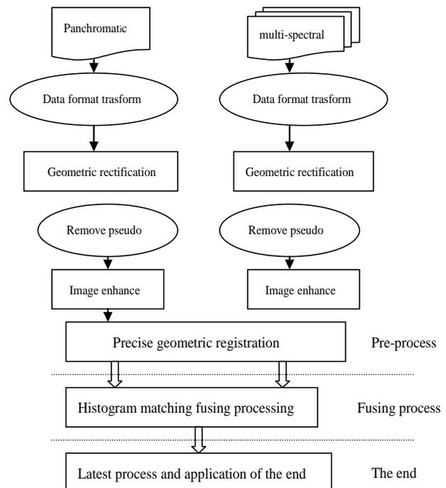
Figure 1 Basic procedure of image fusion between multi-spectral images and panchromatic images
