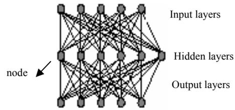
Figure 1. Multi – layer perceptron model
