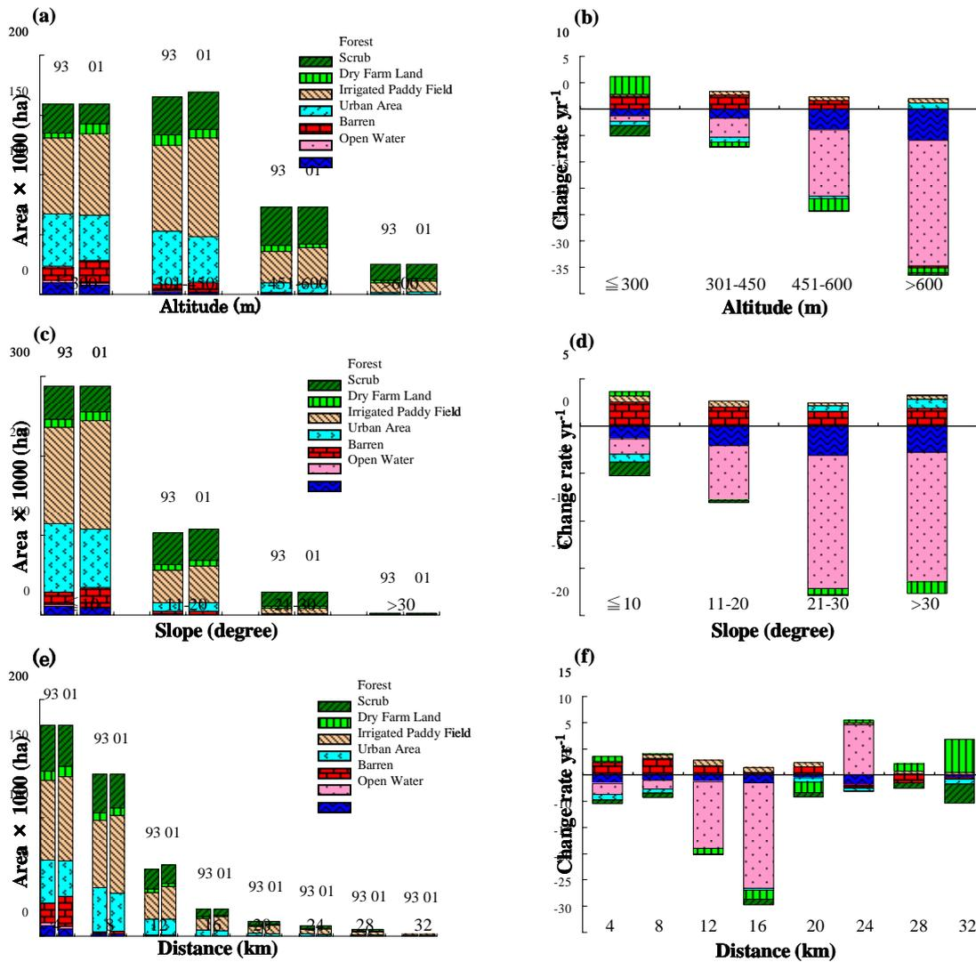
Figure 2. Results of change detection by using characteristic datasets: (a) landcover distribution between 1993 and 2001 by altitude and landcover type; (b) landcover changes by altitude; (c) landcover distribution between 1993 and 2001 by slope and landcover type; (d) landcover changes by altitude; (e) landcover distribution between 1993 and 2001 by distance and landcover type; (f) landcover changes by distance
